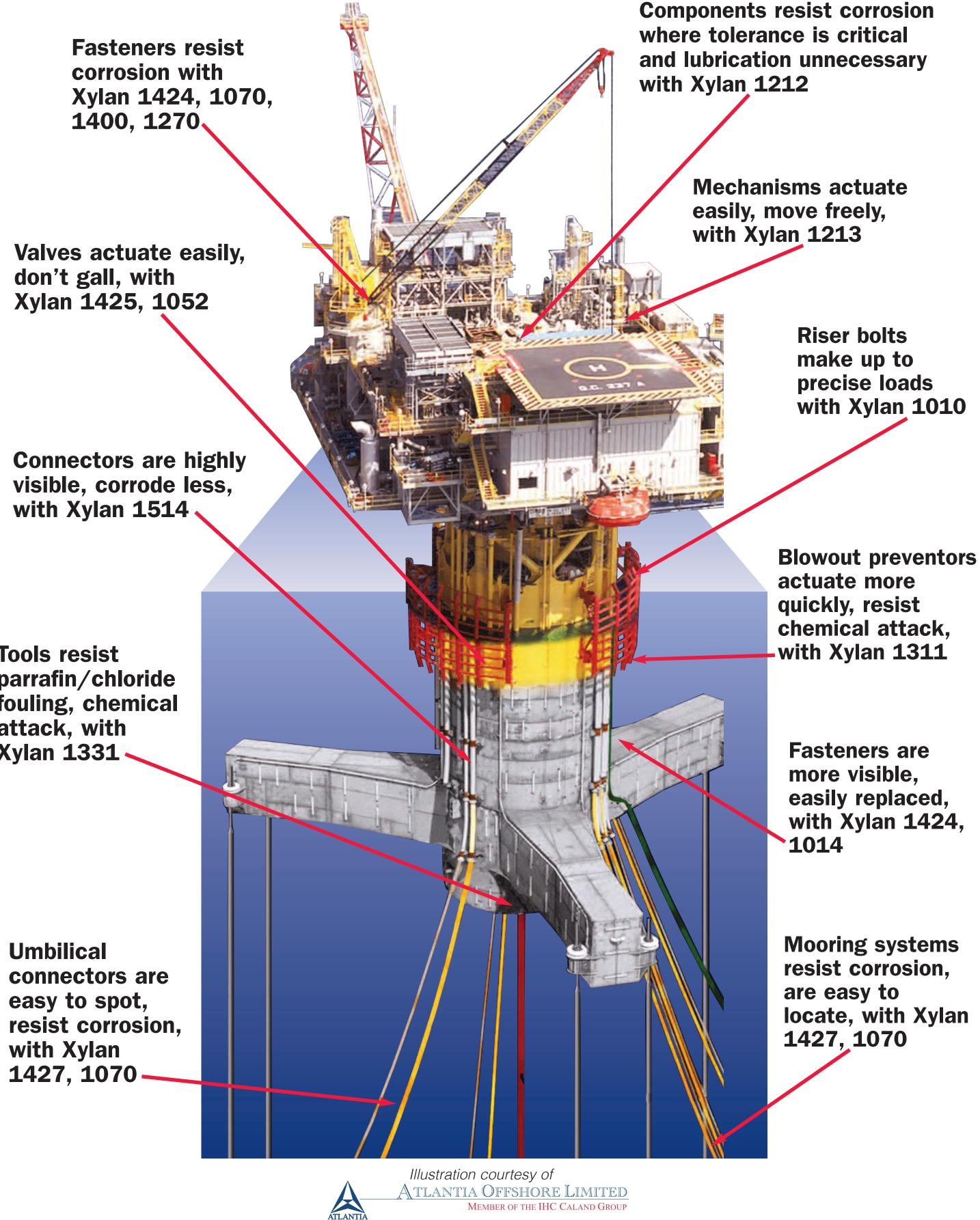
**Tools resist** parrafin/chloride fouling, chemical attack, with Xylan 1331
